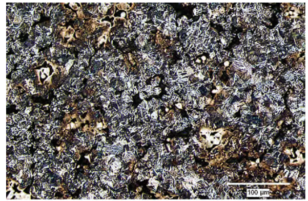
Figure 4: MPIF FL 4405, carbonitrided, microstructure; white halos surrounding pores are nitride layer
