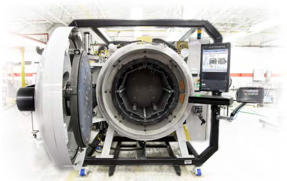
The Titan® vacuum furnace is one of Ipsen's global modular platforms
