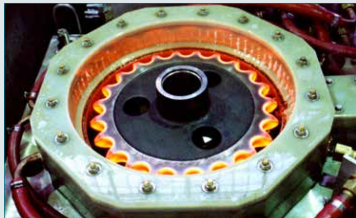
Fig. 2: Typical Single Shot Induction Hardening Operation. [Photograph Courtesy of Ajax-Tocco-Magnethermic]
