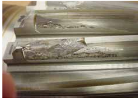
Figure 3: Severe pitting from end loading.
