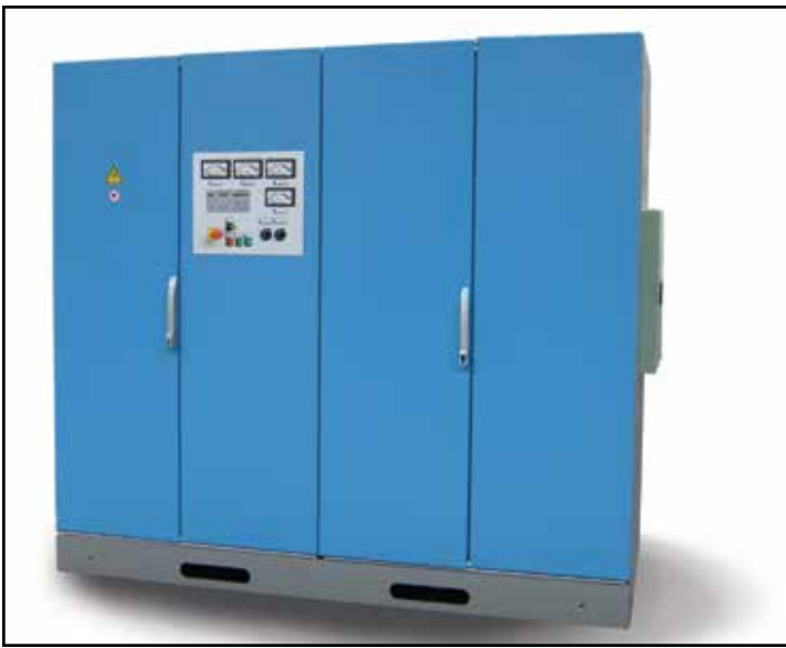
Figure 3: Inductoheat's STATIPOWER IFPT is a novel IGBT-type power supply specifically designed for induction hardening and tempering applications allowing independently adjustable frequency via CNC-program in a 5-40kHz frequency range and power in the range of 10-360kW
