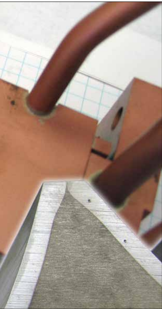
Figure 1 (left): In tooth-by-tooth hardening, inductors can be designed to selectively harden specific areas of gear teeth where metallurgical changes are required [2]
