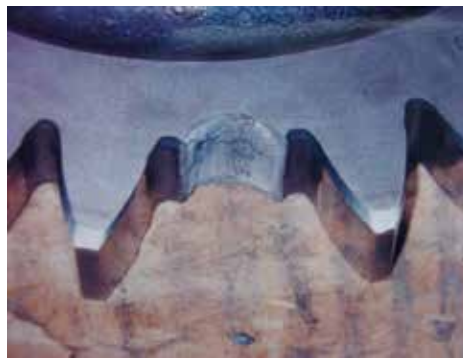
Figure 1: Tooth damage due to bending fatigue.
