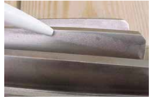
Figure 4: Soft spots in the carburized case (Observed After Shot Peening).
