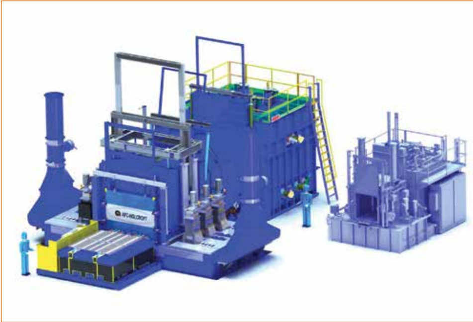
Figure 1: An illustration of the physical size difference between the Monster™ UBQA and a standard UBQ integral quench batch furnace with a 3,500 Lb. [1,588 Kg] load size of 36" w x 48" l x 36" h.
