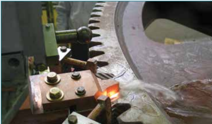
Fig. 3: Tooth-by-Tooth Induction Hardening –Process. (Photograph Courtesy of Ajax-Tocco-Magnethermic)
