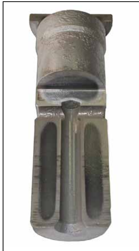
Figure 9: Carrier pin – simultaneous OD and ID hardening. (Courtesy of ERS Engineering Corp.)
