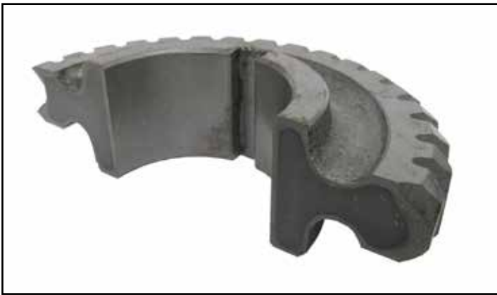
Figure 7: Section of the induction hardened transmission gear. (Courtesy of ERS Engineering Corp.)
