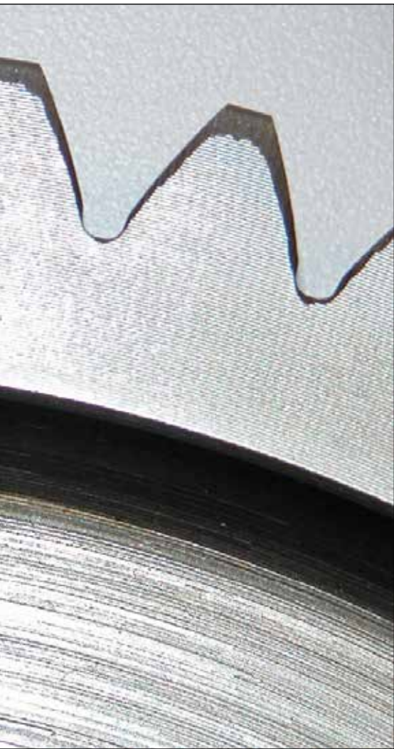
Figure 1: Tooth damage due to bending fatigue.
